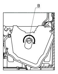
(4) Set the accompanying partition plate and the spacer plate to the position as shown in the figure.
