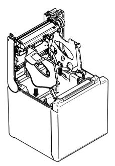
See "RP-E10 SERIES THERMAL PRINTER TECHNICAL REFERENCE" to set the paper width (MS2-6) to 58 mm.
