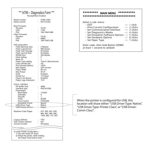
Print Test and Configuration Menu Sample. Samples will vary depending on the printer model. The A799 is LogoEZ® compatible for ease of setting-up your logo and two-color design needs.
