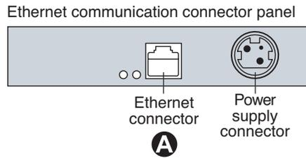
1. You don't need to turn off the computer. Plug the printer end of the Ethernet cable into the Ethernet connector port on the printer (A). Make sure the connector snaps firmly in place.
