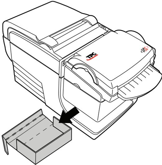
Remove and save the cardboard supports from the slip path after you have placed the printer in its user position.
