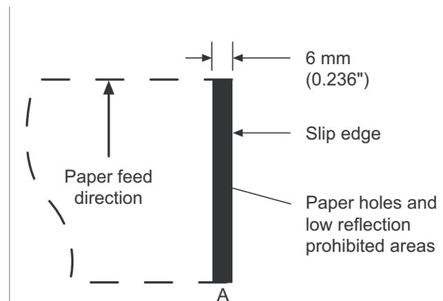
The Slip sensors that activate the slip-in light use a reflective photo sensor.
