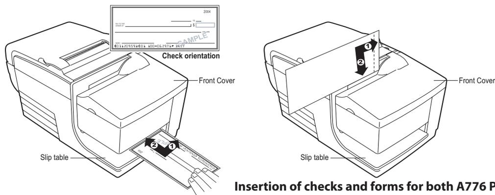
**Insertion of checks and forms for both A776 Printers**
