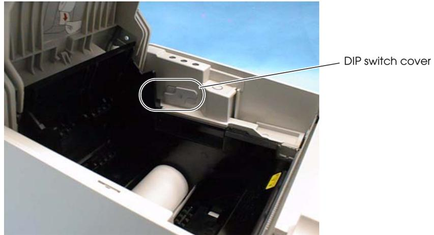
Before setting DIP switches, remove the DIP switch cover.
