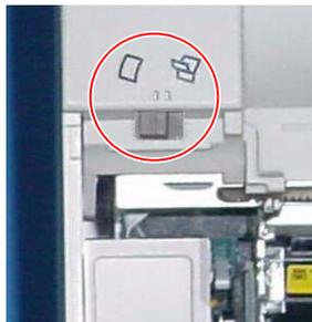
6. As shown in the following figure, pull the end of the paper to the bottom of the square hole above the manual cutter (label peeling sensor).
