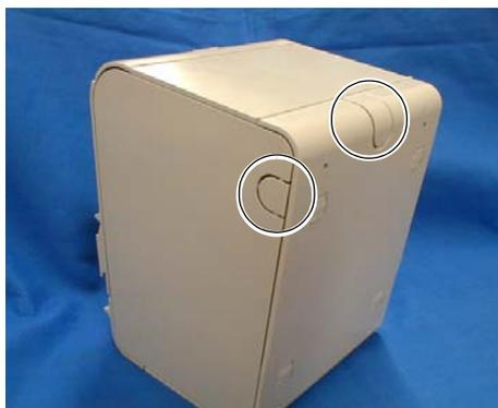
3. Remove the bottom of the cover as shown in the illustration below.
