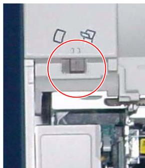
7. As shown in the following figure, pull the end of the paper to the bottom of the square hole above the manual cutter (label peeling sensor), and close the roll paper cover.
