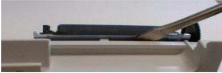
*Adhesive being removed with flat-blade screwdriver*
