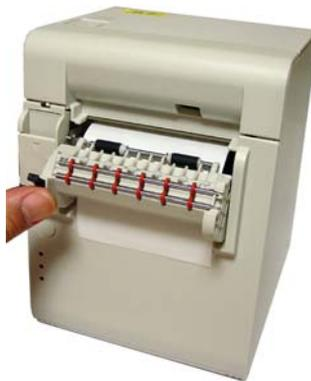
10. Press FEED. The printer automatically feeds the paper to the start position, and the PAPER OUT LED goes off.
